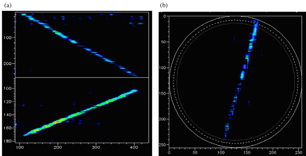
**Figure 3.** A cosmic muon event in 1 bar of  $\text{CF}_4$ : (a)  $xz$  projection (top),  $yz$  projection (bottom) and (b)  $xy$  projection. The binning is 3.5 mm for  $x$  and  $y$  and 1.7 mm (80 ns for  $z$ ).
