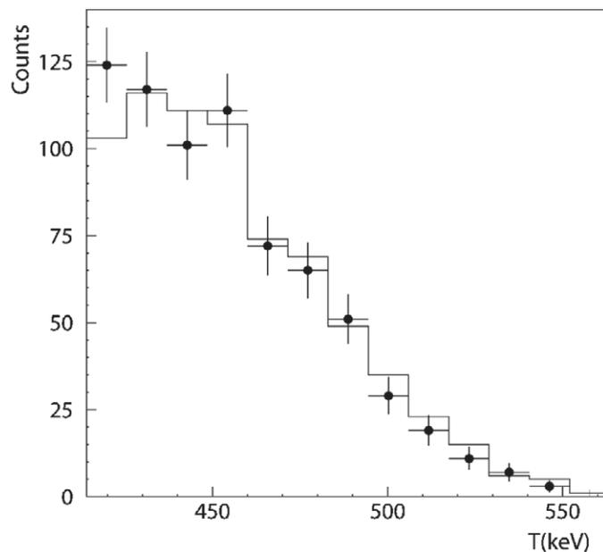
**Figure 2.** A Compton spectrum of  $^{137}\text{Cs}$  in the TPC compared with Monte Carlo simulation (filled circles).
