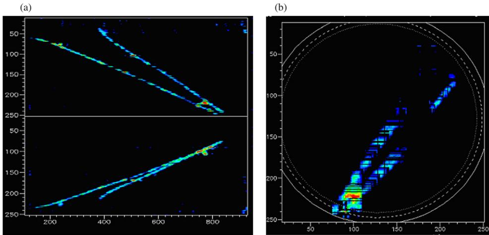
**Figure 5.** Two  $e^+e^-$  pairs: (a)  $xz$  (top),  $yz$  (bottom) and (b)  $xy$ .
