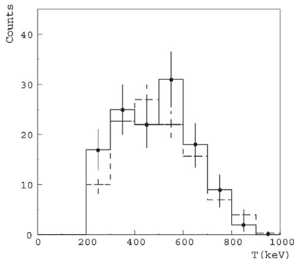
**Figure 10.** Energy spectrum of forward (solid line with filled circles) and NB (dashed line) electrons.
