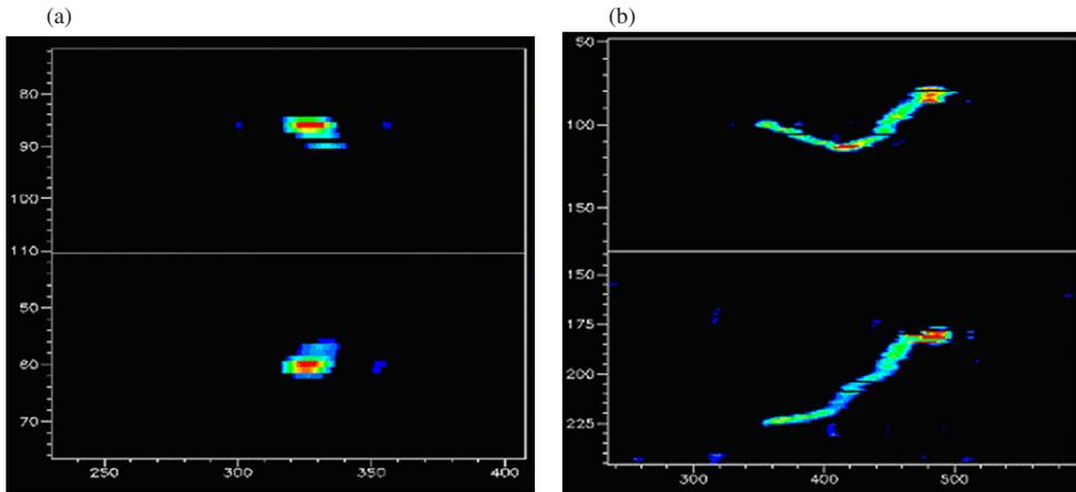
**Figure 7.** Low energy single electrons of (a) 80 keV (4.5 cm) and (b) 540 keV (35 cm) at 1 bar in the TPC:  $xz$  (tops) and  $yz$  (bottoms).
