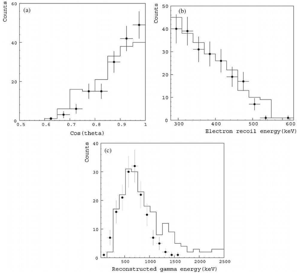
**Figure 12.** (a) Scattering angle  $\theta_{\text{source}}$ , (b) electron recoil energy  $T_e$  and (c) reconstructed gamma energy  $E_\gamma$  (c) for  $^{137}\text{Cs}$ , compared with Monte Carlo simulations (filled circles).
