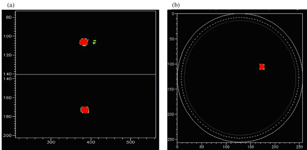
**Figure 4.** An alpha particle event: (a)  $xz$  (top),  $yz$  (bottom) and (b)  $xy$ .
